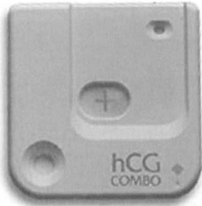
FIGURE 44 Two-antibody diagnostic assay (pregnancy, Abbott's TestPack TM ) printed using continuous ink-jet technology.
