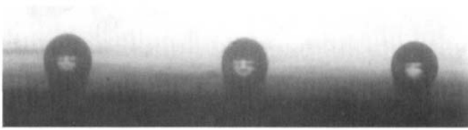
FIGURE 25 Profile view of 65- \mu\text{m} -diameter hemispherical microlenses printed onto the tips of single-mode fibers within a fiber array.
