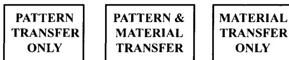
FIGURE 5 The major classes of pattern and material transfer technologies. If self-assembly is possible, only the material needs be transferred because it intrinsically contains the information (instructions) to spontaneously form structures.
