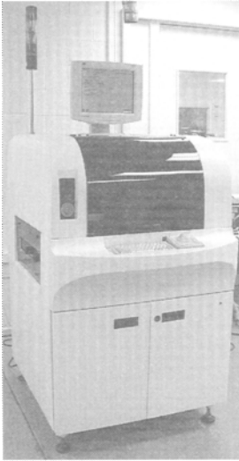
FIGURE 12 The overall system provides a work area of 12" × 12". This size work area is ideal for board manufacturing, boats/carriers and individual components. The overall footprint of the system is 36.5" × 47" × 59.5" and will ultimately incorporate multiple material capability for electronic and biological materials (courtesy Optomec, Inc., Albuquerque, New Mexico).
